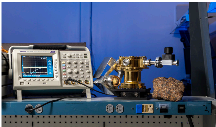
The LLNL team designed and built the gamma-ray spectrometer for the NASA mission to Psyche over five years from 2018 to the spring of 2023.
