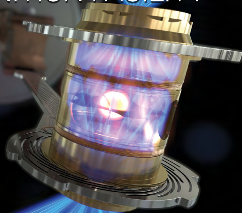
The decades-long quest to achieve fusion ignition and energy gain in a laboratory setting culminated with a NIF experiment that applied 2.05 MJ of laser energy to compress a capsule of deuterium-tritium fuel and produced 3.15 MJ of fusion energy.
